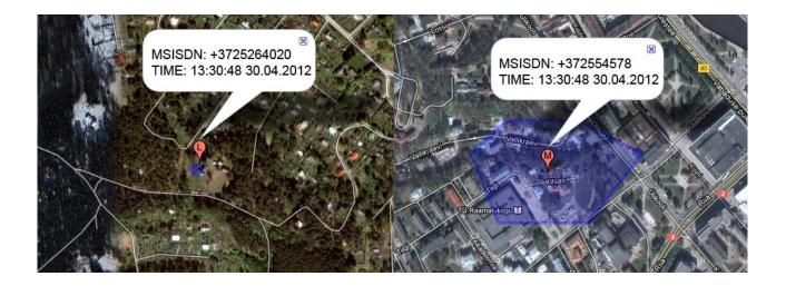
GPS precision (accuracy: ~10 m) and 3G MPS (~200 m using trilateration)
